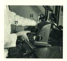
7. Disconnect the jet block driving rod connecting rod yoke from the type carrier cam lever extension by removing the screw and the yoke position pin. Replace the pin and screw in the yoke, after disconnection, to avoid loss.
