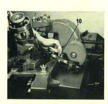
5. Unhook the actuating lever link (10) from the fusing stop on the mould and disconnect the elongated eye from the pin on the actuating lever. Remove the link from the machine.
