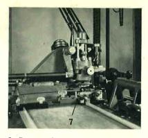
3. Remove the matrix holder (7) from the matrix lifter. Disconnect the air nozzle holder, air nozzle and collar, and the crossblock oiler from the main stand by removing the long screw and its washer.
