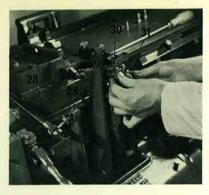
10. Connect the type pusher lever connecting rod ball stud (28) to the type pusher cam lever (29), securing with the nut.
