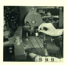
7. Unhook the weight (13) from the ratchet pin chain and lay it on the shelf inside the main stand, convenient for reconnection.
