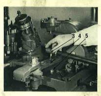
2. Disconnect the mould blade slide drive lever connecting tube ball end (3) from the intermediate lever (4) by removing the locking nut (5). Replace the nut on the ball end to avoid loss.
