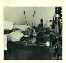
6. Remove the mould oiler from the mould.
