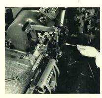
15. Grease the locating faces of the mould water supply piping, and with one end on the main stand stud, swing into place and finger tighten the nut (40). Screw into the mould, and then further tighten the nut with a wrench.
