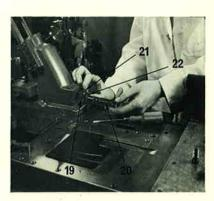
8. Bring the mould blade slide (19) forward to expose completely the mould blade fork (20). Free the connecting pin by a half turn anti-clockwise of the locking screw (21), and then remove the pin (22) to disengage the fork. It is important to ensure that the head of the lock screw is not left protruding above the face of the mould blade slide, or it will be damaged when the slide is withdrawn.
