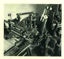
14. Grease the locating faces of the mould water supply piping (41) marked 'A.B.' and attach to the main stand stud. Screw the piping to the mould and then affix the washer and nut to the main stand stud.
