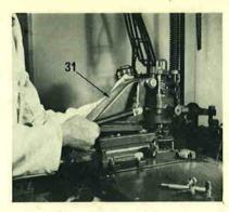
11. Assemble the composition matrix head (31) on the matrix heads base, locating the keyways over the keys on the base. Secure in position with the one long screw and the three shorter screws.
