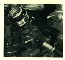
12. Position the mould on the adaptor base and secure it with the locating screw. Position the low quad lever for either high or low product, and connect the spring plate to the mould blade lever. Screw the type clamp operating block to the adaptor base.
