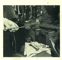
8. With the stop lever handle (21) in the low position marked *Leads*, turn the plunger spring adjusting nut anticlockwise so that the spring will exert only minimum pressure. Set the fulcrum pin at the 1—3 L and R position.
