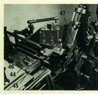
14. Close up the adjustable type channel block (44) to the fixed block (45), and secure to the type carrier cover with the screw and washer (46). Grease the locating faces of the mould water supply piping (47), and connect the piping to the mould. Attach the mould oiler to the mould (not shown), and insert the matrix holder complete with a matrix into the matrix lifter.
