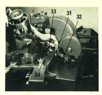
11. Attach the actuating lever link (31) by placing the elongated eye (32) over the pin on the actuating lever, and connecting the hook (33) at the other end to the fusing stop (34) on the mould.
