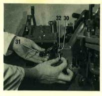
10. With the mould blade slide (30) in the forward position, attach to it the appropriate mould blade fork (31). Insert the connecting pin, and twist until it is felt to grip; at this point, tighten the set screw (32).
