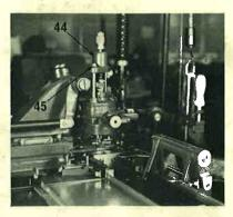
16. Sorts casting for large type composition will require the use of the centring pin auxiliary loading spring bridge (44) instead of the loading spring bridge normally in position on the composition matrix head.
