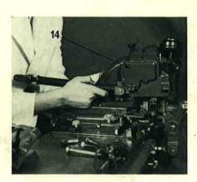
5. Remove the four screws securing the display matrix head (14) to the base. Take a firm grip on the head and lift it off the machine.
