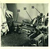
11. Attach the composition matrix head (32) to the matrix heads base and secure with three screws and the one long screw. Connect the matrix lifter lever connecting rod (33) to the top hole of the matrix cam lever (34) with the rod eye pin and nut.
