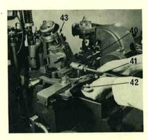
16. Connect the lower pump body lifting spring plate by the upper hole to the swing frame post.
