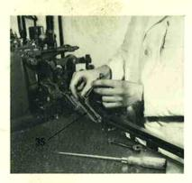
12. Fit the furniture guide (35) to the main stand, using the cutter blade bracket screw, the collar, long screw and washer. Release the lead clamp and insert a piece of product of the required size into the mould.
