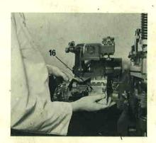
5. Turn the machine to 20°, and remove the product from the mould. Place the mould blade slide in the forward position so that the blade connection of the 1—3 point mould, or the connecting pin for the 4-18 point mould, is clear of the wedge housing. The pin may be removed at this point, and the set screw tightened to prevent damage.
