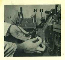
Substitute, if necessary, the mould blade fork (23) already connected for the one suitable for the product to be cast.
