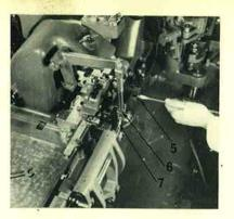
3. Remove the screw securing the water supply piping (5) to the mould, and remove the nut and washer securing the other end of the piping to the main stand stud. Take off the piping.
