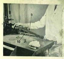
4. Remove the two screws and washers securing the lead stacker bar (9) to the lead stacker (10), and lift it off. The lead stacker bar does not need to be taken off the machine except for the production of Furniture.
