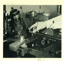
3. Disconnect the mould blade slide drive lever connecting tube ball end (6), from the intermediate lever (7), by removing the nut (8) and lifting the ball end free. Replace the nut onto the ball end and swing the tube clear of the intermediate lever.
