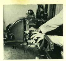
12. Turn the machine to 200° and place the mould blade slide in the backward position.
