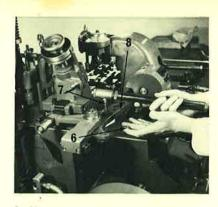
3. Unscrew the lock nut (6) and disconnect the mould blade slide drive lever connecting tube ball end (7) from the furniture position on the intermediate lever (8).
