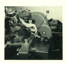
5. Take off the actuating lever link (13) by unhooking it from the fusing stop on the mould, and releasing the eye from the fin on the actuating lever.
