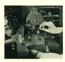
6. Unhook the weight (14) from the ratchet pin chain of the counter bracket. Disconnect the actuating rod eye from the actuating lever (15) by removing the pin (16). Re-connect the lower hole of the rod eye to the rod housing with the same pin. Loosen the machine.
