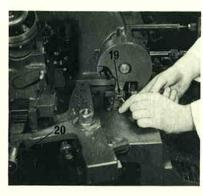
6. Detach the weight from the ratchet pin chain, and disconnect the actuating rod eye (19) from the actuating lever by removing the pin. Use the same pin to connect the lower hole of the rod eye to the actuating rod housing.
