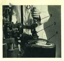
2. Fit the pump (3), nozzle (4) and piston (5) required for the change of product, so that the parts have time to attain the working temperature whilst the change-over is being made.
