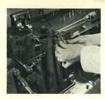
9. Remove the nut securing the type pusher lever connecting rod ball stud to the matrix cam lever, and disconnect the type pusher lever (23) from the cam lever (24). Replace the nut on the ball stud.
