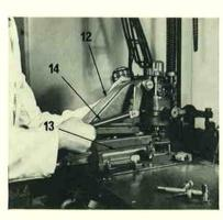
6. Remove the Composition matrix head (12) from the matrix heads base (13), by disconnecting the matrix lifter connecting rod (14) from the matrix cam lever, and removing the three short screws and one long screw.
