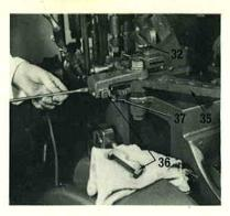
11. Pull the intermediate lever (35) to the left to disconnect it from the plate (36), and then change the plate for the one marked *Furniture* by removing the two screws.
