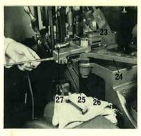
11. Place the stop lever handle (23) in the low position. Slacken off the spring adjusting nut. Set the fulcrum pin at the 1—3 L and R position.
