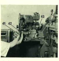
13. Connect the lead clamp intermediate lever rod yoke (41) to the lead clamp lever with the pin. Replace the clip (42) over the pin to secure in position.
