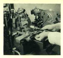
2. Remove the mould oiler piping and support from the underside of the mould oiler by releasing the knurled nut.
