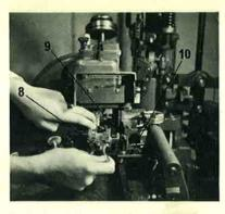
3. Remove the matrix holder (8) from the display matrix head, by pulling the small release lever with the fingers of the left hand, and withdrawing the holder with the right hand. After casting quotations, ensure that the matrix lifter handle is returned to its normal position by raising the lock pin knob on top of the matrix head.
