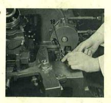
7. Remove the pin to disconnect the actuating rod eye from the actuating lever (18). Connect the rod by the lower of the two holes to the rod housing, using the same pin as before.
