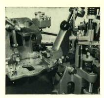
12. Bring the jet block driving rod forward so that its hook (31) is clear of the counter bracket. This will make it easier to locate the hook on the jet block in position over the hook on the driving rod when the mould is assembled on the machine.
