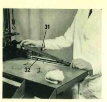
9. Attach the lead stacker bar (31) to the lead stacker (32), with the two screws and washers already in position on the stacker.
