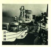
12. Secure the composition mould to its adaptor base; place the low quad leverspring lever in the required position, and connect the spring plate (36) to the mould blade lever. Place the type clamp block in position and secure with its two screws.
