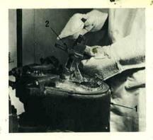
1. Switch off the electric motor; turn off the water supply; and place the gear control in the neutral position. Lower the pot (1) and if necessary, change the pump body (2) and nozzle so that they will be hot enough for casting when the change-overhas been completed. These parts will be too hot to handle with safety unless adequate protective material is used.
