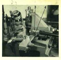
2. Disconnect the mould blade slide drive lever connecting tube ball end (3) from the intermediate lever (4), by removing the stud nut from the underside of the lever and lifting the ball end out of the hole. Move the tube to one side so that it is clear of the top of the machine.
