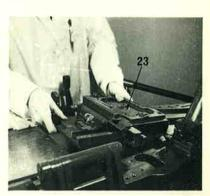
8. Place the matrix heads base (23) in position on the main stand, locating the keys in the keyways. Check that the locating key distance piece (24) (see picture 9) is in the correct position for 5—36 point. Secure the matrix heads base to the main stand using the three base screws.
