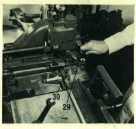
11. Place the mould blade slide in the forward position and attach the mould blade fork, of the required point size, with the pin. Turn the pin clockwise until it grips and then tighten the screw.
