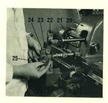
7. Assemble the counter bracket (20) to the main stand, locating the keys in the keyway. Insert the four screws to secure the bracket to the machine.
