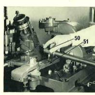
15. Connect the spring plate by the upper of the two holes to the swing frame post. Connect the mould blade slide drive lever connecting tube ball end (50) to the hole marked *Leads* on the intermediate lever (51).
