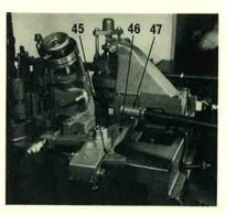
16. Set the eccentric lever fulcrum pin (45) on the mould blade slide drive lever (46) to the required position marked 5—36 type.
