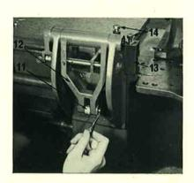
5. Disconnect the cutter actuating plunger link (11) from the cutter actuating lever (12) by removing first the split pin and then the cutter actuating pin.
