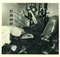
15. Place the stop lever handle (37) in the uppermost position. Turn the eccentric fulcrum pin to indicate the required point size of type. Check that the driving block cap abutment is set for the set size of type to be cast, i.e. for set sizes above 12 point the large diameter end should be towards the rear of the machine.
