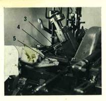
2. Disconnect the Mould Blade slide drive lever connecting tube ball end (3) from the intermediate lever (4), by removing the nut (5) from the ball end and lifting the tube clear. Replace the nut onto the ball stud to avoid loss.
