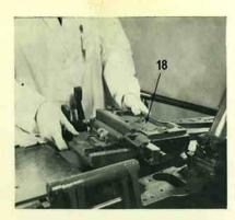
9. Place the matrix heads base (18) in position on the main stand, locating the keys in the keyways. Check that the base locating key distance piece is in the required point size position, and reverse if necessary.
