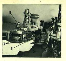
3. Remove the air nozzle and holder; the crossblock oiler, and the mould oiler. Disconnect the mould water supply piping (5), and after releasing the knurled lock nuts remove the mould blade fork pin with a pin handle (6).
