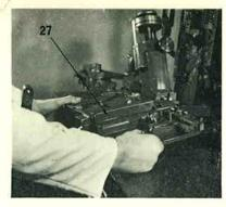
10. Take out the three screws which hold the matrix heads base to the main stand. Grasp the matrix heads base (27) firmly in both hands and lift it off, complete with the type pusher lever connecting rod and the type carrier connecting rod. Wipe the main stand clean.
